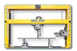
The motor unit is driven in force or displacement, and then it is possible to apply a predetermined stress or to impose to the structure a displacement.
