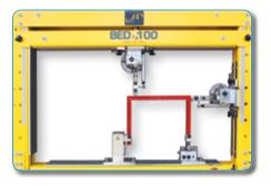
The user can decide to measure a force, a moment, a displacement relating to load in several points of the structure.
